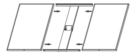
Slide the two solar panels (black side face up) from either side of our fitted bracket. Installation diagram After aligning the screw holes on both sides, lock the fixing screws (PA6\*16 screw\*4pcs fixed).
